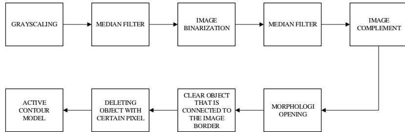
Fig 4. Preprocessing flow diagram
